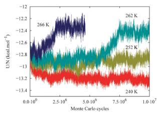
**Fig. 2** Plot of the total potential energy (U) per particle from the liquid- $I_h$  direct coexistence simulations of the quantum system at p = 1 bar.
