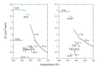
**Fig. 4** Molar volume change ( $\Delta v = v_{\rm B} - v_{\rm A}$ ) along the phase boundaries from (Left) path integral simulations and (Right) experimental results (w indicates the liquid phase).<sup>1</sup>
