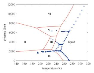
Fig. 3 Phase diagram of water from path integral simulations of the TIP4PQ/2005 model. Experimental results (blue points) are also shown.  $^{1,56}$
